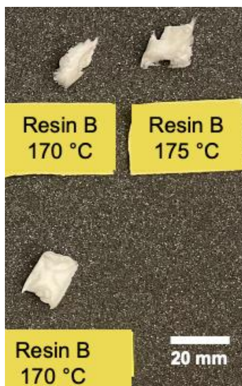
Figure S1. Photograph of Resin B foamed at temperatures above its end melting point under Method 1 (top) and Method 2 (bottom).
