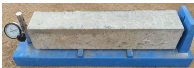
(a) Shrinkage testing of a UHPC specimen
