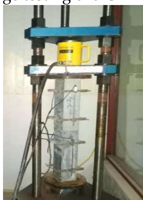
(b) Creep testing of a UHPC specimen
