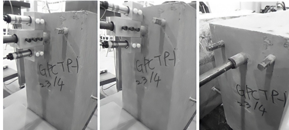
Figure 3. Front face images of plain bar reinforced GPC specimens: photos taken before ( left ), during ( middle ) and after ( right ) the beam end test.
