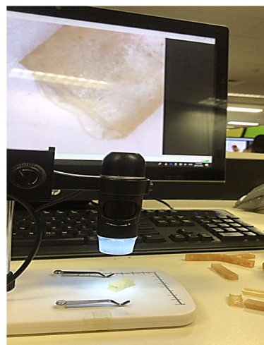
Figure 7. Microstructure Analysis (A Digitech® 5MP USB Microscope Camera).
