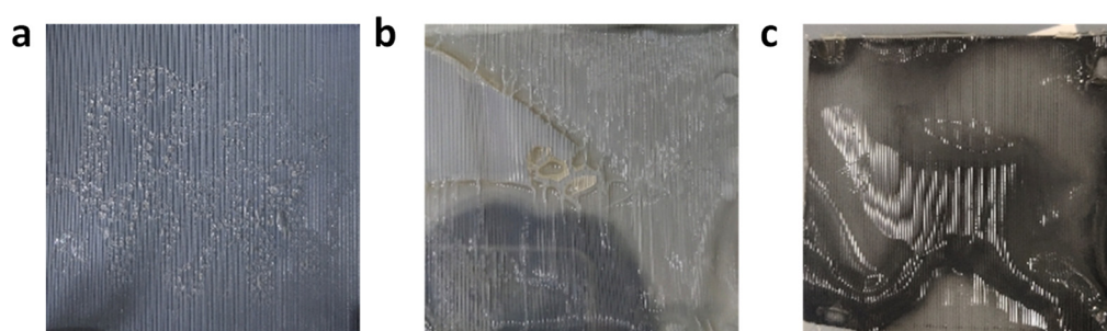
Figure S1. The photos of composite membranes by one-step coating way with (a) 5 wt% cast solution, (b) 10 wt% cast solution, and (c) 20 wt% cast solution.
