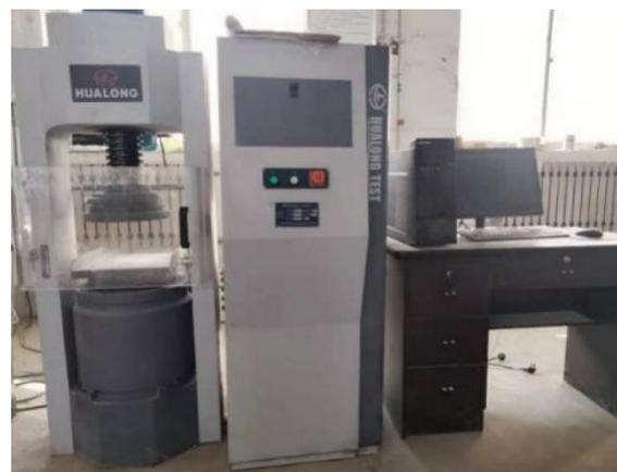
**Figure 3.** The testing apparatus of the cube compressive and splitting tensile test.
