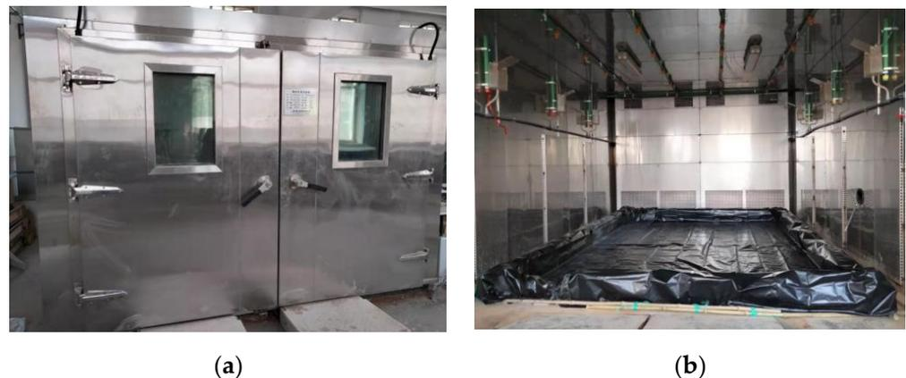
**Figure 2.** The environmental simulation test chamber. (a) Overall appearance; (b) Internal structure.
