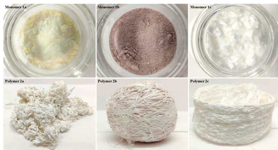
Figure 1. Photographic images of the thiol-functionalized norbornene dicarboximide monomers ( top ) and their corresponding ROMP-prepared raw polymers ( bottom ).
