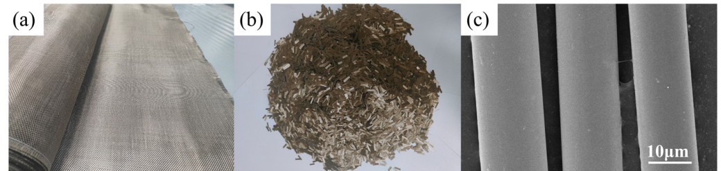
Figure 3. Shape and appearance of BF, (a) BF sheet, (b) short-cut BF, and (c) scanning electron microscopy image of BF.
