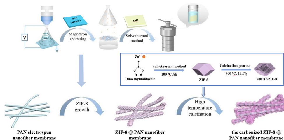
Figure 1. Fabrication route of the carbonized ZIF–8@PAN nanofiber membrane.
