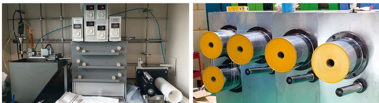
Figure 2. Lab-scale wet-spinning and drawing equipment.
