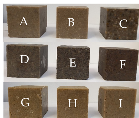
Figure 6. Samples (A–I), particle-reinforced composites, samples: (A–C) with different filler sizes (more in Table 1), (D–F) with different short fibre volume and same fillers (more in Table 2), and (G–I) with different epoxy resins and constant fillers mixture (more in Table 3).
