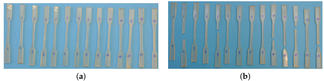
Figure 1. Specimens used in tensile and creep tests: (a) prior to testing, (b) after testing.
