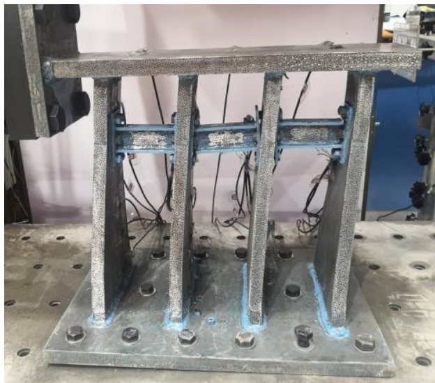
Figure 9. Deformation of the specimen \Delta = 100 mm.
