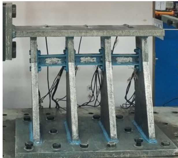
Figure 7. Deformation of the specimen during loading.
