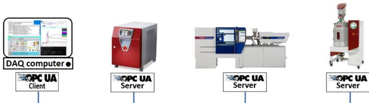
**Figure 2.** OPC UA communications platform to collect data from injection molding machine and peripherals.
