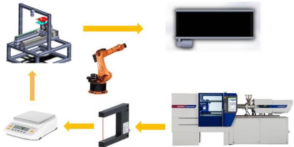
**Figure 7.** The procedure of handling and measurement of the injection molded part [5].
