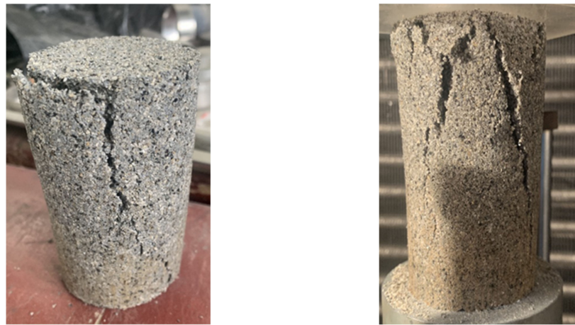
Figure 3. Samples after UCS test for (a) without wet–dry cycles and (b) with wet–dry cycles.
