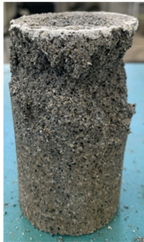
Figure 6. Sample stabilized by composite stabilizer after UCS test.
