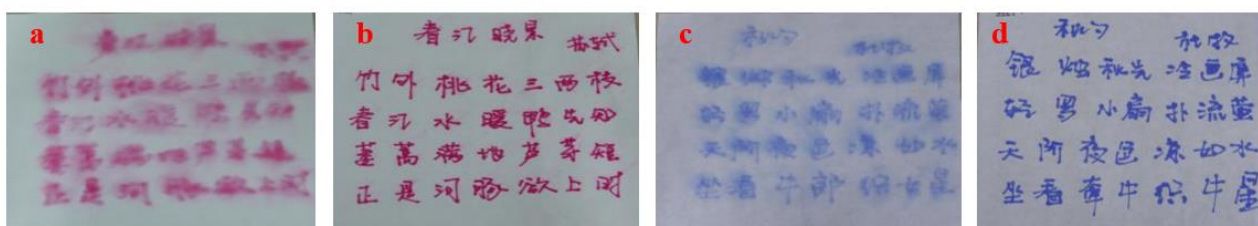
Figure 12. Pictures of paper with red and blue ink handwriting after lining technology: (a,c): untreated; and (b,d): treated with HACC nanoparticles.
