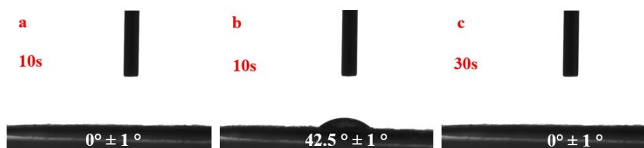
Figure 10. Contact angle of Xuan paper samples before and after coated with HACC nanoparticles: (a) uncoated paper after 10 s; (b) coated paper after 10 s; and (c) coated paper after 30 s.
