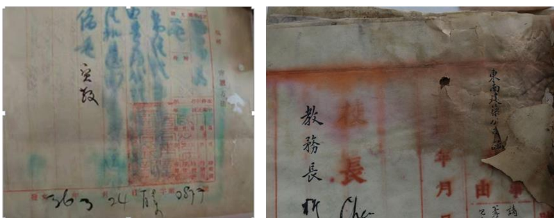
Figure 1. Typical example of blue ink (left) and red ink (right) migration of 19th century documents.
