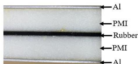
**Figure 10.** The cross-section of the beam used for the natural frequency testing.
