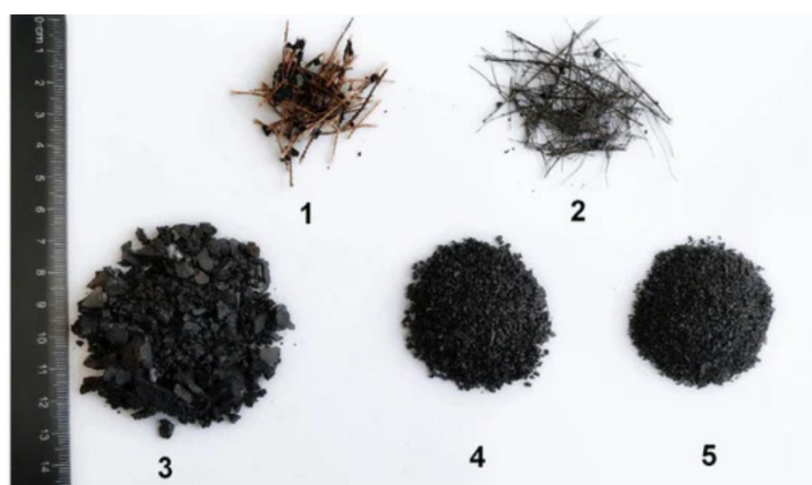
Figure 1. The different materials extracted from end-of-life tires such as (1) textile fiber, (2) metal cord, (3) large size fraction of rubber crumb (1–5 mm), (4) mean size fraction (1–2 mm), and (5) small size fraction (0.1–1 mm) [15].
