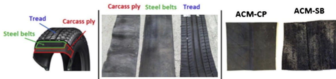
Figure 13. Description of the tire parts used for the development of the ACM systems based on carcass ply (ACM-CP) and steel belts (ACM-SB) [29].
