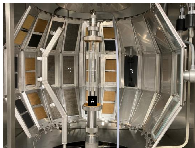
Figure 3. Example of test frame placement in Xenon-arc weathering meter. The letters “A”, “B”, and “C” represent the xenon-arc lamp, the black panel thermometer, and the test frame with two yarn specimens, respectively.
