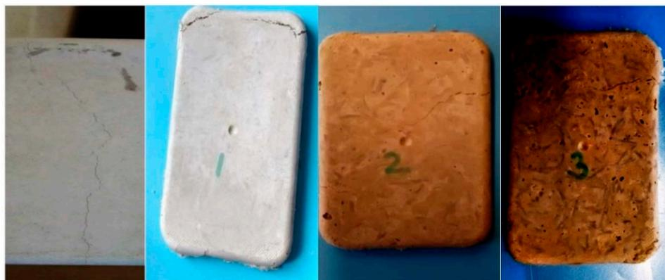
**Figure 10.** Crack patterns in 0%, 1%, 2%, and 3% basalt-fiber-reinforced concrete samples after tensile testing (pictures formatted so that crack patterns are clearer).
