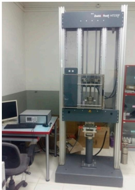
**Figure 2.** Zwick/Roell universal tensile tester.
