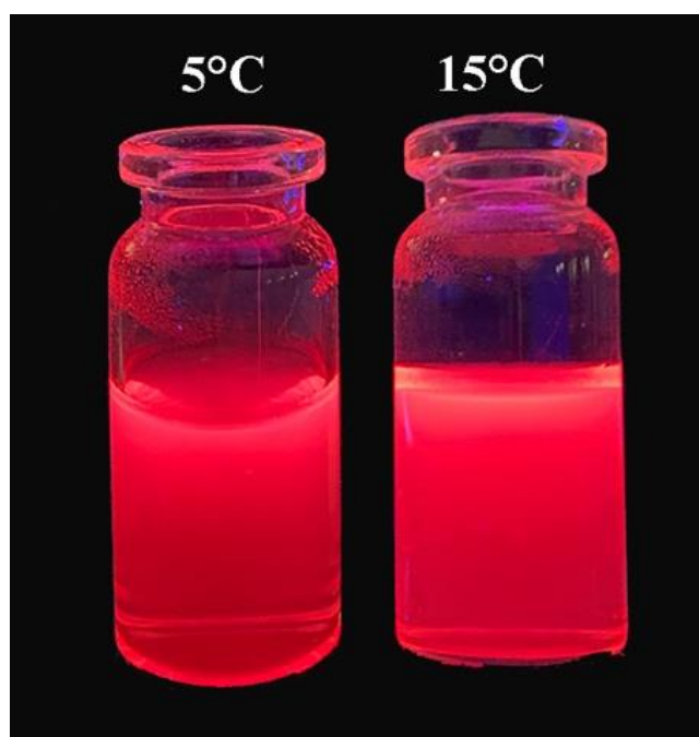
Figure S1. AuNCs solution at 5°C and 15°C under UV lamp illumination.
