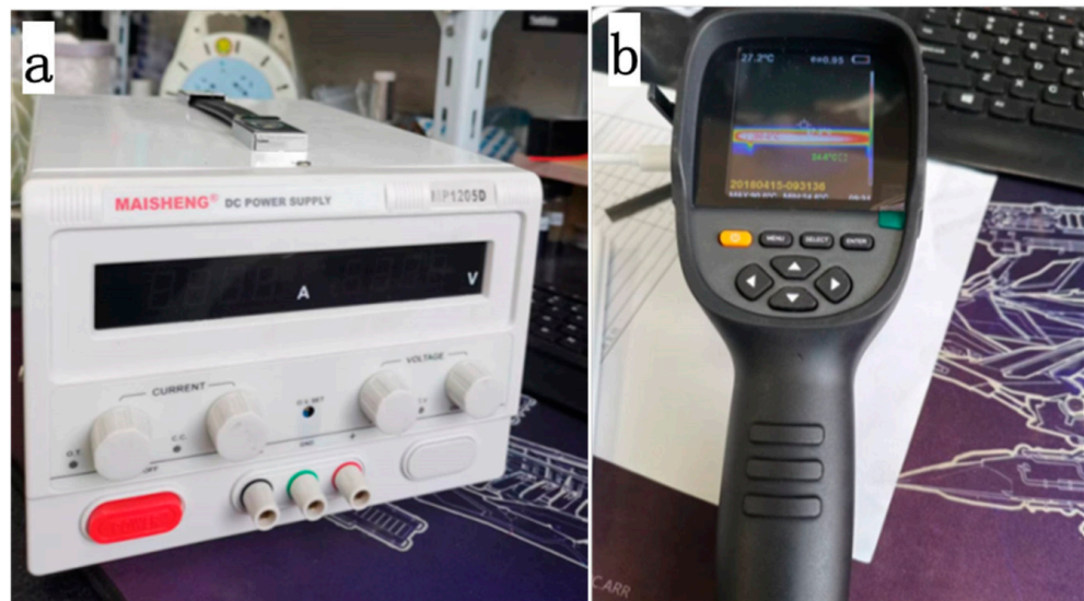
Figure 2. (a) The DC power supply, and (b) the infrared thermal imager.
