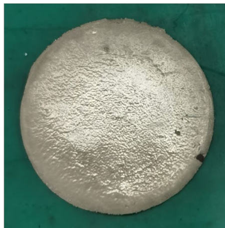
Figure S7. Photo images of the bare Cu foil and the \text{ZnF}_x(\text{OH})_y@\text{Cu} foil after Li deposition at 6.0 \text{ mAh cm}^{-2} .
