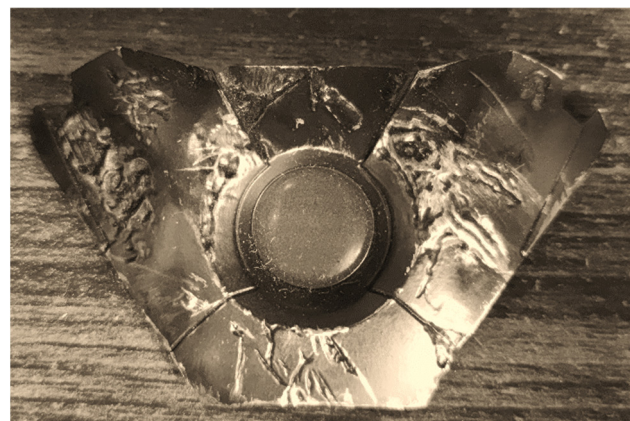
Figure 5. Actual Battle Damage Distribution of Armor.
