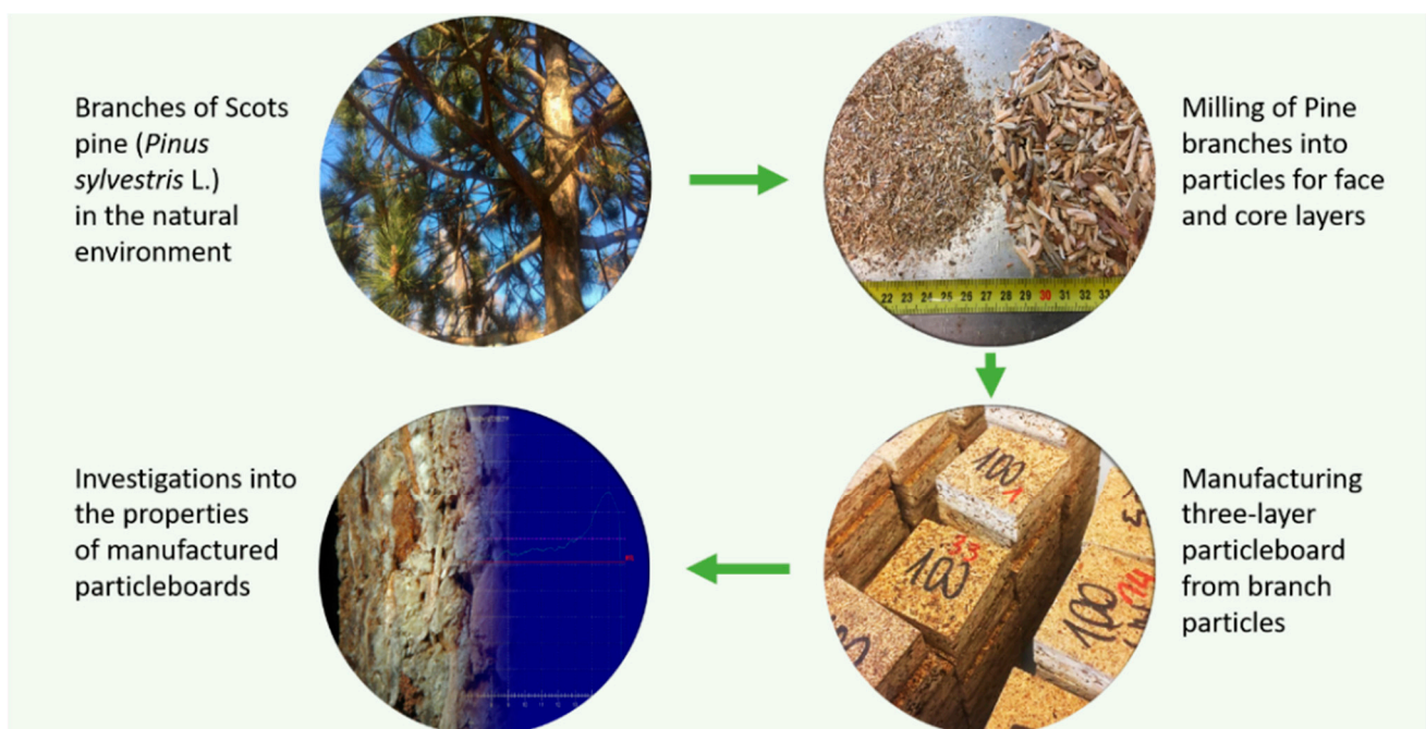
Figure 2. The general production process of three-layer particleboard from pine branches.
