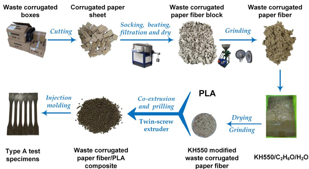
Figure 1. Preparation process diagram of the WCPF/PLA composite.
