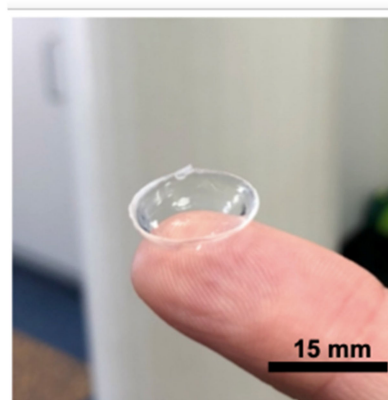
Figure 2. A prototyped soft contact lens from COC moulds after cleaning and swelling on a finger for scale.
