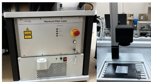
Figure 1. Installation for nanoparticles synthesis by laser ablation: laser-mechanical unit (left) and stand with galvano-mechanical scanner (right).
