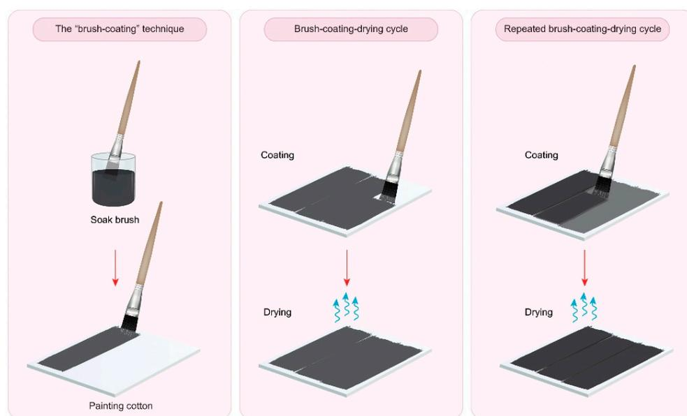
**Figure 1.** Diagram of “brush-coating-drying” technique.
