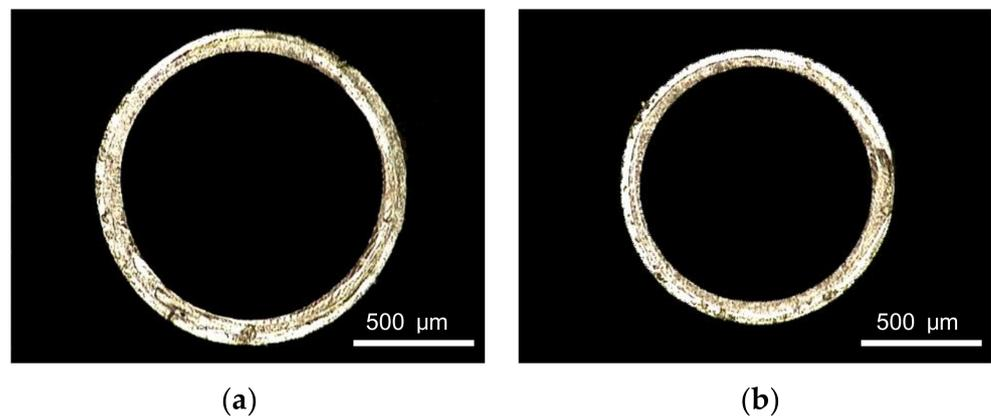
**Figure 10.** Cross section of micro tubes at different pulling speeds: (a) Pulling speed = 7 m/min; (b) Pulling speed = 12 m/min.
