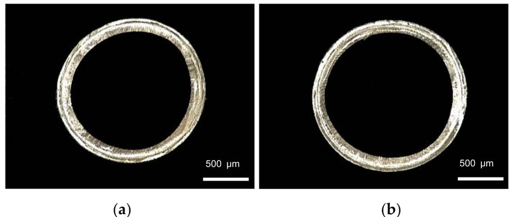
**Figure 17.** The cross section of micro tubes at different vacuum degrees: (a) Vacuum degree = 0 inH<sub>2</sub>O; (b) Vacuum degree = 45 inH<sub>2</sub>O.
