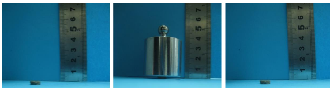
Figure S4. A GIA 1 with a weight of 6.4 mg (left); the same sample supporting a 200g poise (middle) that is 31250 times its own weight; the same sample after remove of the poise (right).
