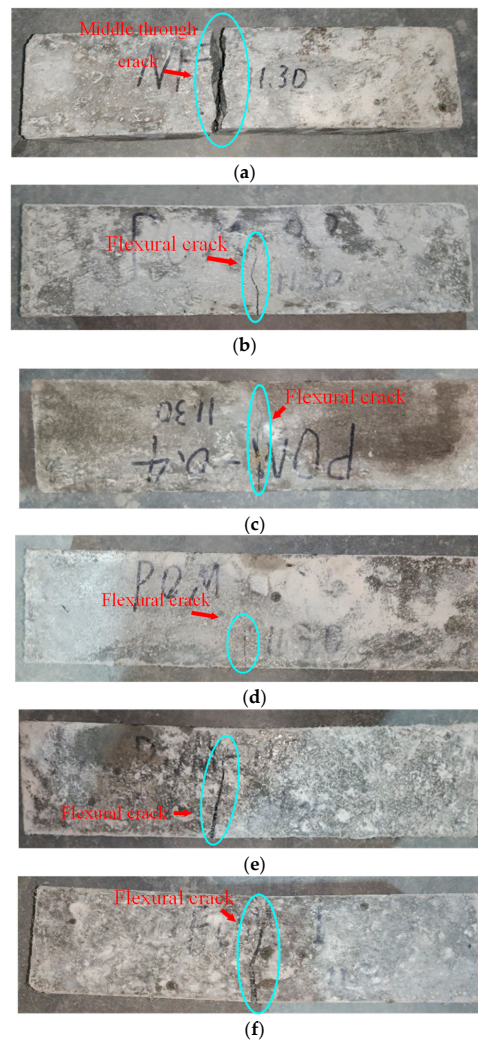
Figure 24. Failure performance of flexural tests: (a) NF; (b) POM-0.2; (c) POM-0.4; (d) POM-0.6; (e) POM-0.8; (f) POM-1.
