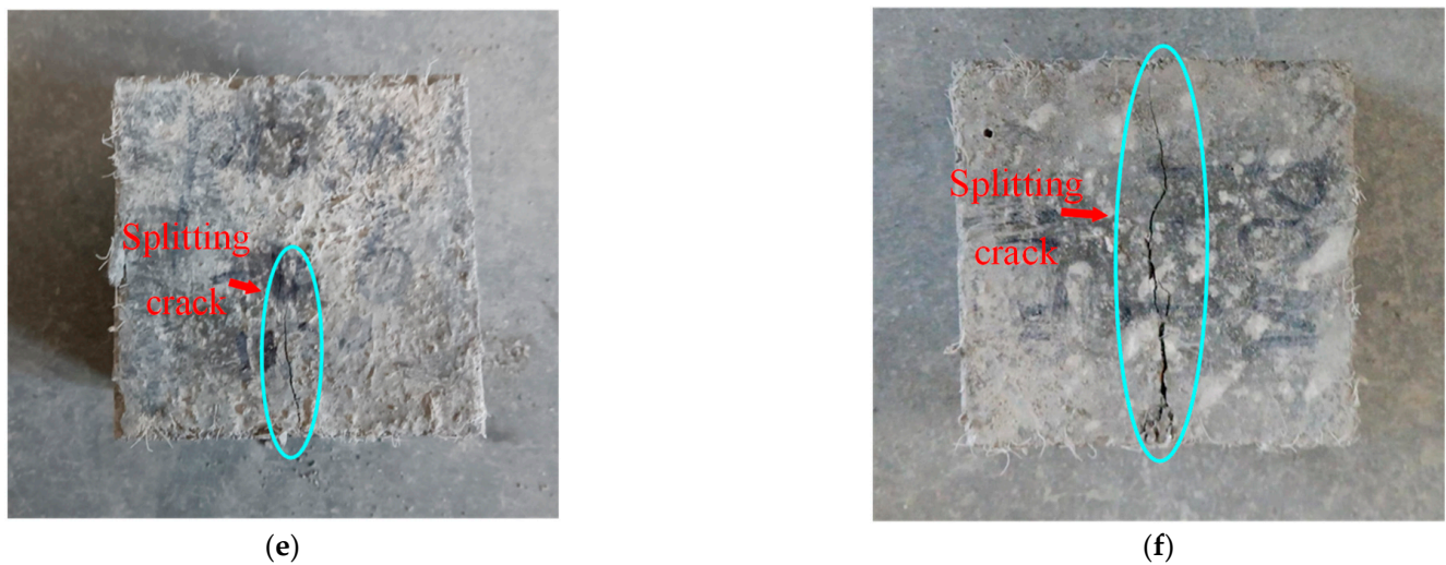
Figure 20. Failure performance of splitting tensile tests: (a) NF; (b) POM-0.2; (c) POM-0.4; (d) POM-0.6; (e) POM-0.8; (f) POM-1.
