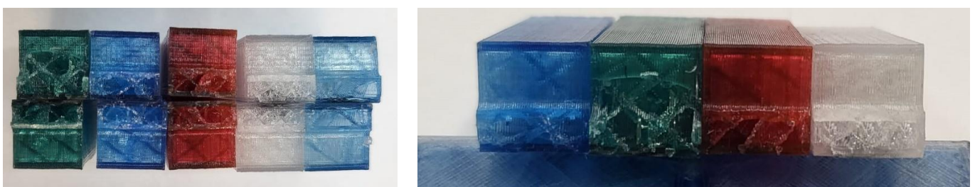
Figure 21. Charpy test specimens.
