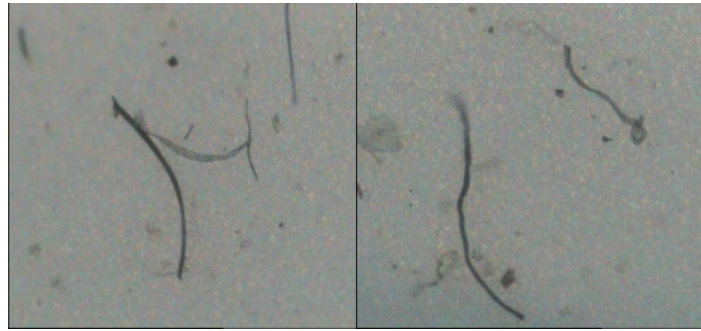
Figure 8. Fibers released from woven fabrics.
