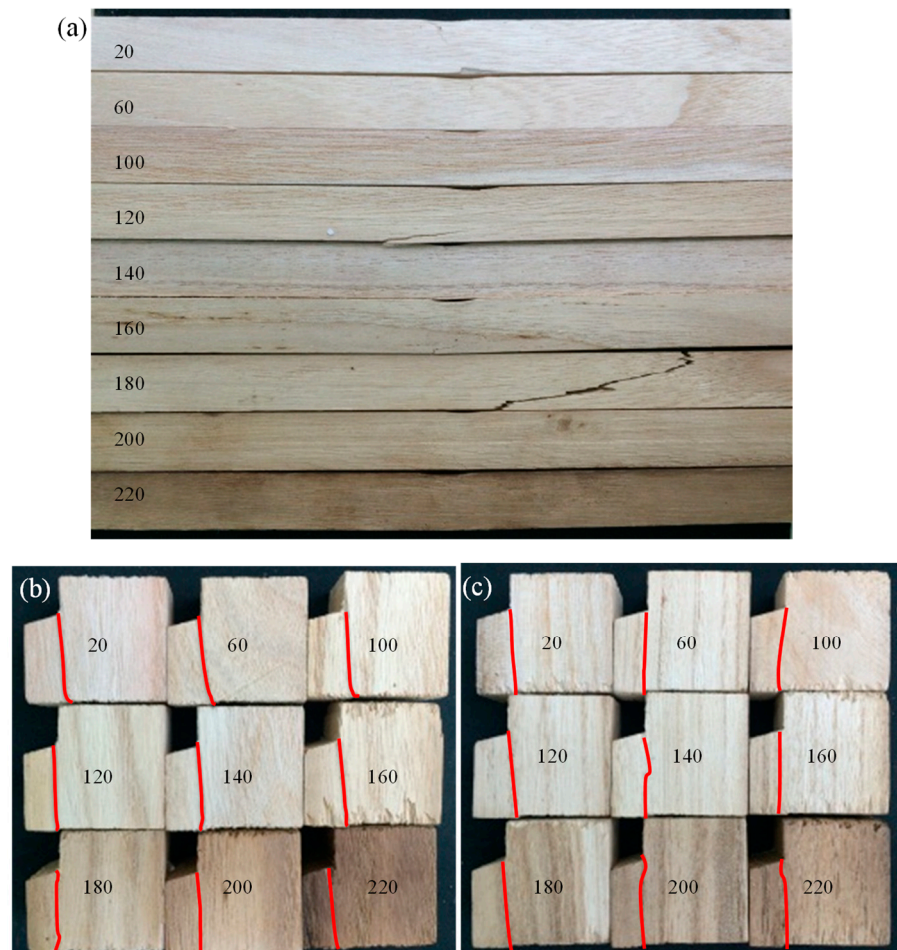
Figure 3. Appearances of the specimens after (a) bending, (b) tangential shear, and (c) radial shear failures.
