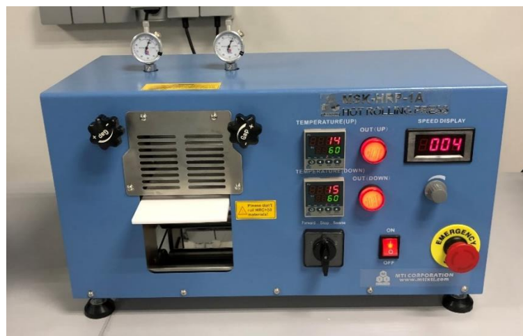
Figure 4. Equipment used for the hot press rolling of solid polymer electrolytes.
