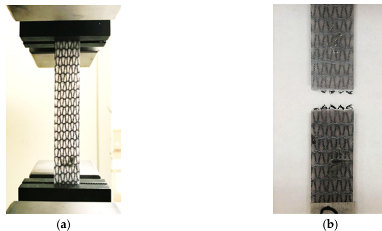
Figure 5. (a) The weft-knitted carbon fiber/polypropylene composite specimen during the tensile test and (b) a tested specimen.
