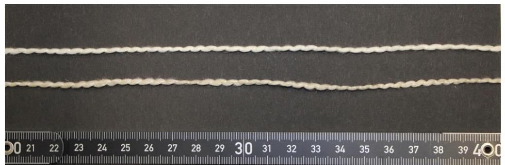
**Figure 5.** Waste cotton hybrid yarn (above) and waste flax hybrid yarn (below).
