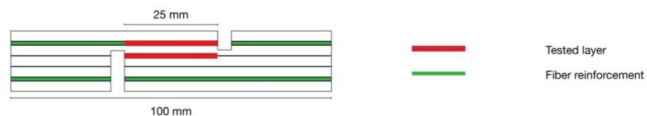
Figure 2. Shear test specimen dimensions of five layered unidirectional reinforced plywood according to EN 314.
