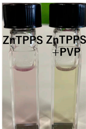
Figure S3. Color change of a 12 \mu\text{M} ZnTPPS solution upon the addition of 0.06 mM PVP.
