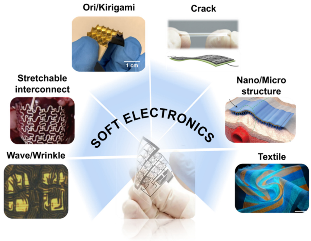
Figure 1. Review summary. Structural design, including wave/wrinkle, stretchable interconnect, origami/kirigami, crack, nano-/microstructure, and textile [13–18].
