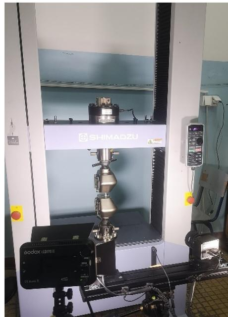
**Figure 3.** Experiment setup for tensile testing using 3D DIC.
