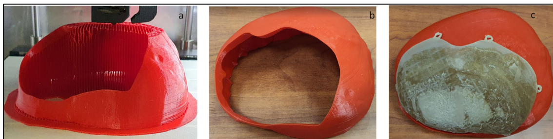
Figure 7. (a) 3D printed skull model of the ABS material with supports, (b) ABS skull model after the removal of the supports, and (c) the rehearsal and fitting evaluation of the PEEK cranial implant on the ABS skull model.
