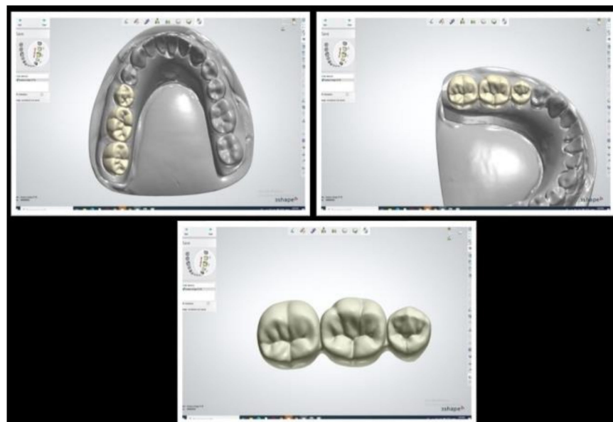
Figure 5. Finished FDP design. Milling the tooth-supported provisional dental prosthesis (group A).
