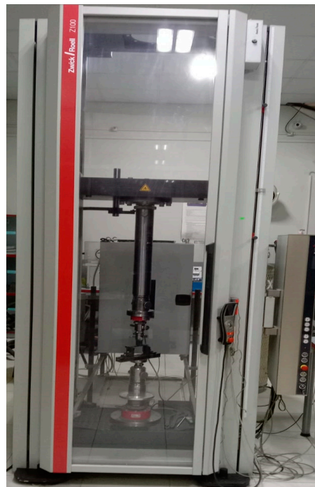
Figure 5. UTM used for the analysis of mechanical properties of the developed composites.
