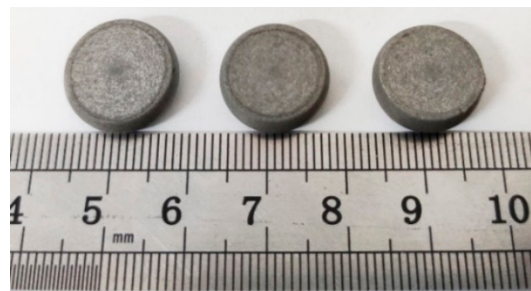
Figure 5. PTFE/Al/Si samples recovered from quasi-static compression test.
