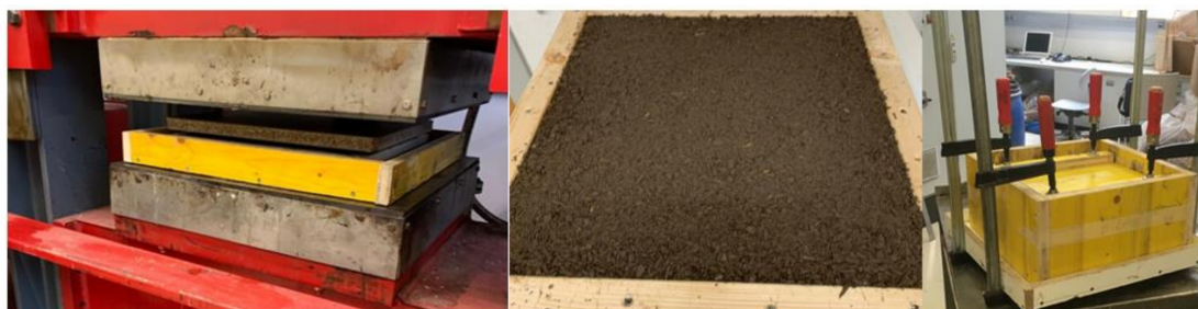
Figure 1. Board compaction by hydraulic press (left); test specimens 430 × 430 × 20 mm in a forming frame (middle); and board compaction by screw clamps (right).
