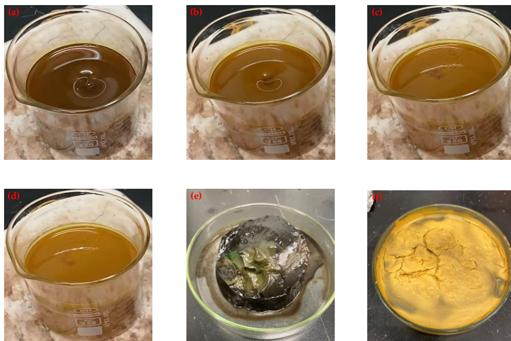
Figure 1. Polymerization mixture of Co-PAM. (a) Initial, (b) 10 min, (c) 20 min, (d) 30 min, (e) after evaporation of alcohol, (f) dry PAM cake prepared without \text{CoCl}_2 .
