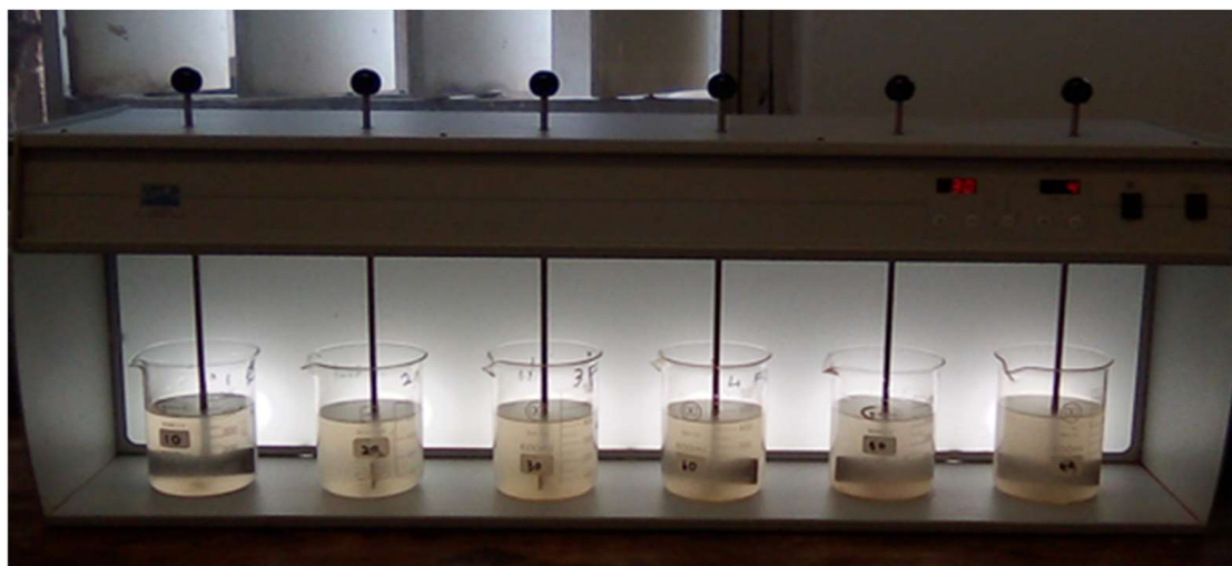
Figure 1. A jar test (JTL6) set-up for the coagulation/flocculation process.
