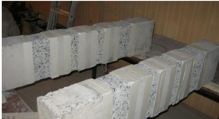
**Figure 2.** General view of the columns, prepared for reinforcement with stirrups and installation of end stirrups-anchors.
