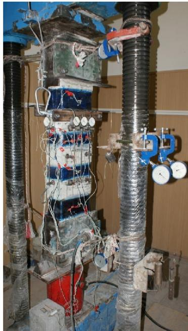
**Figure 7.** The design of the stand for testing columns with the location of mechanical devices and resistance strain gauges for measuring displacements and relative deformations.
