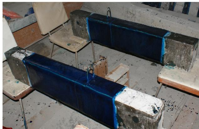
**Figure 6.** General view of the column, reinforced according to the X5 variant—a full clip of three layers of carbon fiber MBRACE FIB CF 300/4900.300 g/5.100 m.
