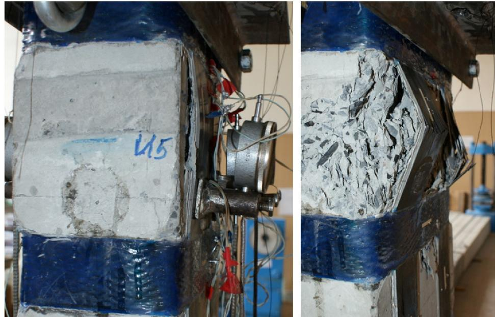
**Figure 11.** Local buckling of the lamellas during the test of the column (5) at a load level in the column of 1100 kN or  $0.8N_{ult}$  (left), at the moment of destruction (right).
